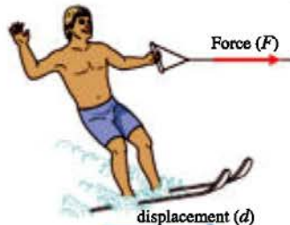
Figure (3): Work done is calculated by the dot product of displacement ( d ) and the force ( F ) acting in the same direction
